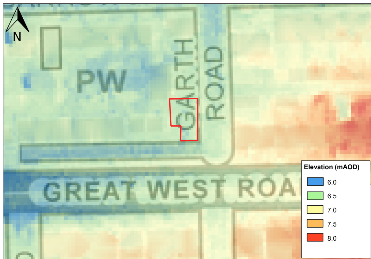
Figure 2 – Site Topography (filtered LiDAR data; site boundary outlined in red)
